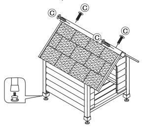
Step 3: Attach roofs and secure with screws.
